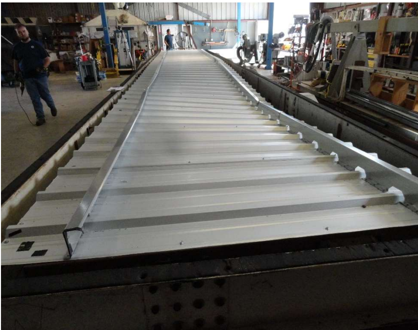
AISI Continuous Span Base Load Test courtesy Roof Hugger
