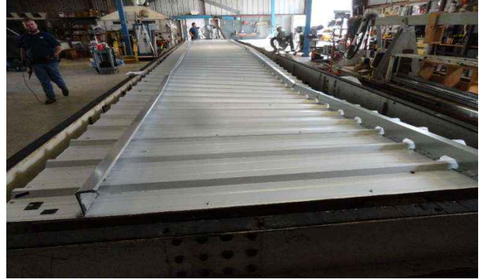
Hugger Continuous span AISI Purlin testing in 50' chamber
