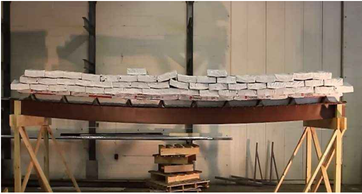
Competitors Non-Industry Standard, Simple Span Test
