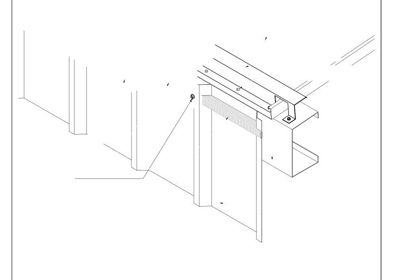
NEW VERTICAL RIB SSR PANEL ROOF OVER EXISTING VERTICAL RIB SSR PANEL ROOF LOW EAVE
