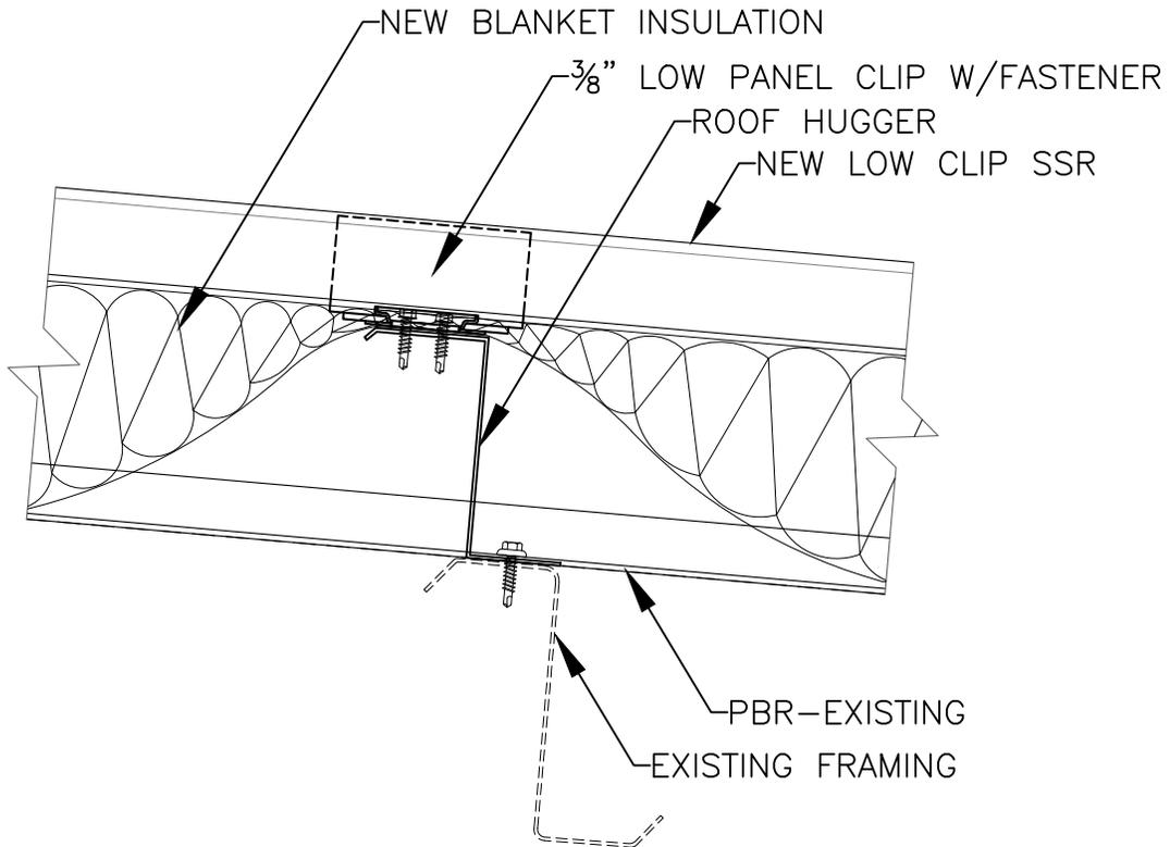
**3/8" LOW CLIP W/NO THERMAL SPACER SSR OVER PBR**
