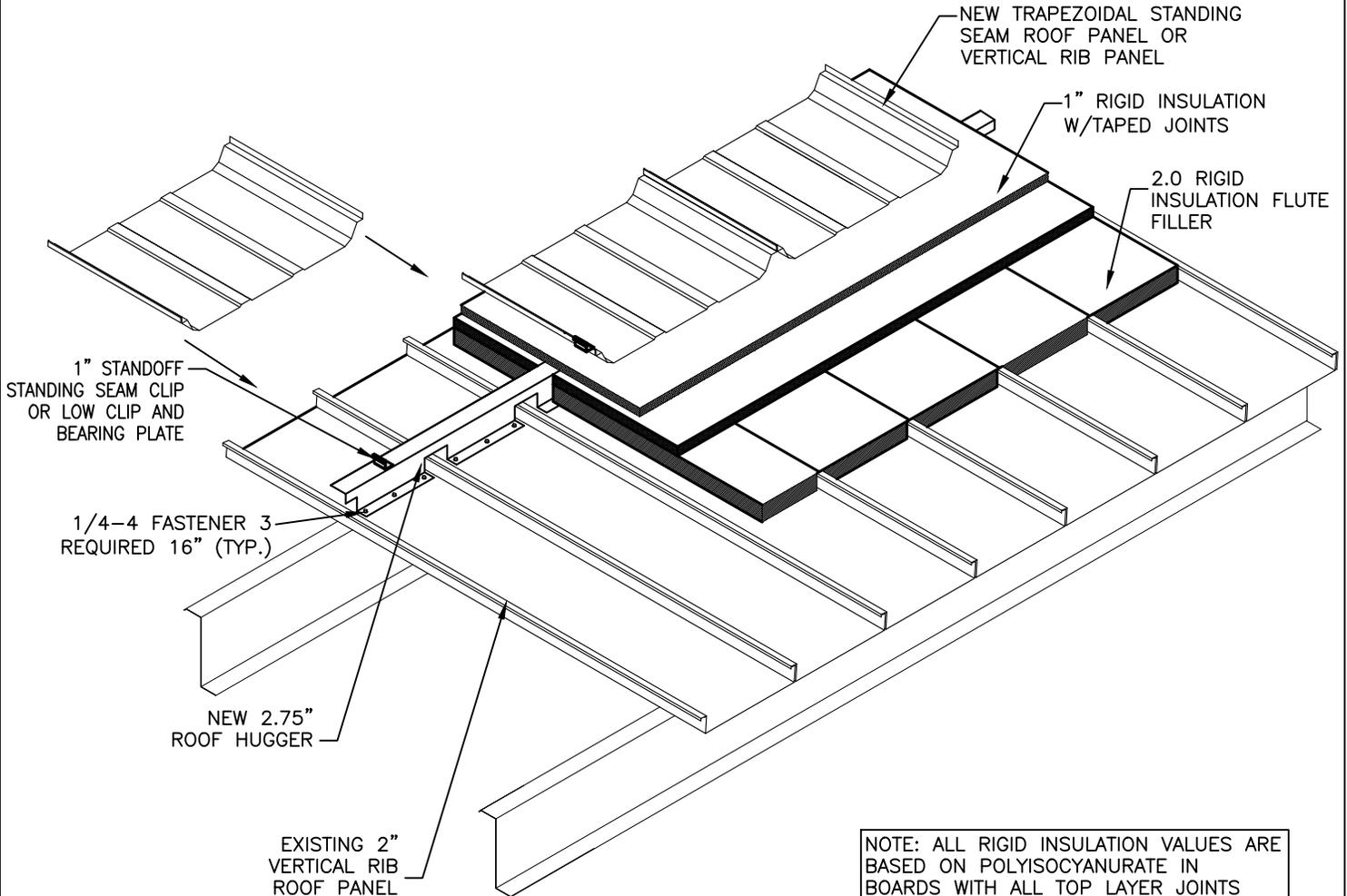
NOTE: ALL RIGID INSULATION VALUES ARE BASED ON POLYISOCYANURATE IN BOARDS WITH ALL TOP LAYER JOINTS AND SEAMS TAPED AND SEALED.
