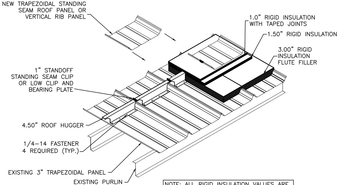
NOTE: ALL RIGID INSULATION VALUES ARE BASED ON POLYISOCYANURATE IN BOARDS WITH ALL TOP LAYER JOINTS AND SEAMS TAPED AND SEALED.
