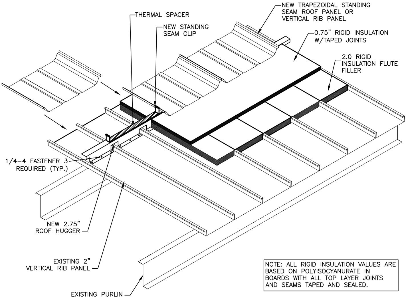
NOTE: ALL RIGID INSULATION VALUES ARE BASED ON POLYISOCYANURATE IN BOARDS WITH ALL TOP LAYER JOINTS AND SEAMS TAPED AND SEALED.
