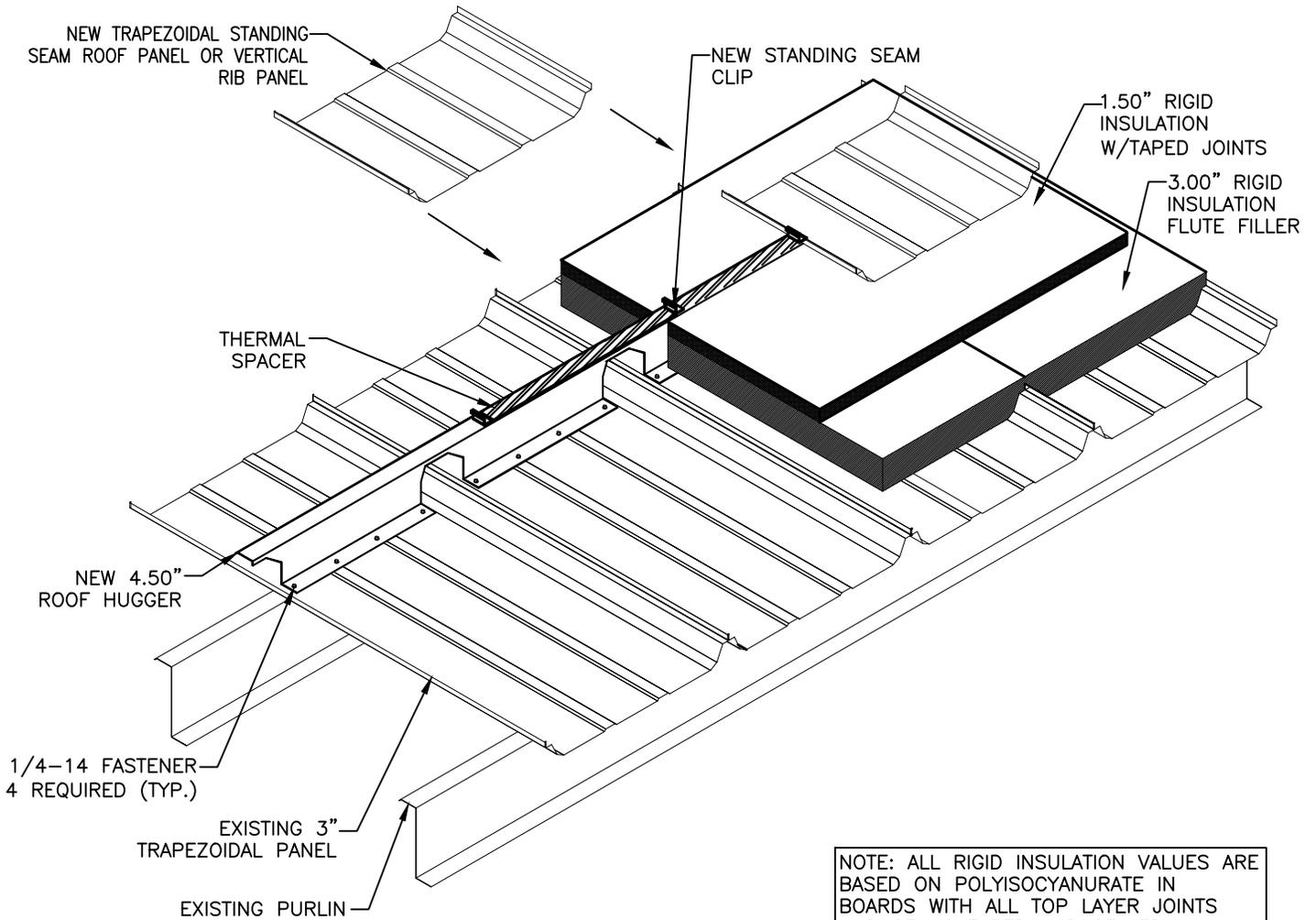
NOTE: ALL RIGID INSULATION VALUES ARE BASED ON POLYISOCYANURATE IN BOARDS WITH ALL TOP LAYER JOINTS AND SEAMS TAPED AND SEALED.
