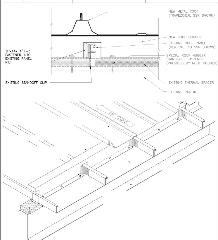
NEW TRAPEZOIDAL SSR OVER EXISTING VERTICAL RIB SSR WITH EXISTING STANDOFF CLIP AND THERMAL SPACER
