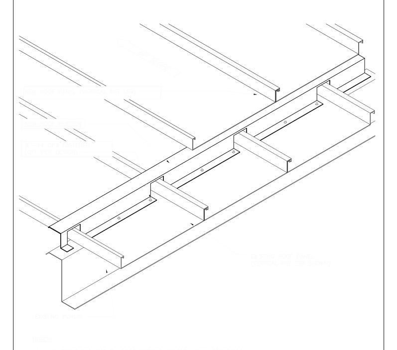
NEW VERTICAL RIB SSR OVER EXISTING VERTICAL RIB SSR WITHOUT STAND-OFF CLIP AND THERMAL SPACER
