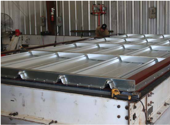
Prior to new panel installation for ASTM E1592 testing
