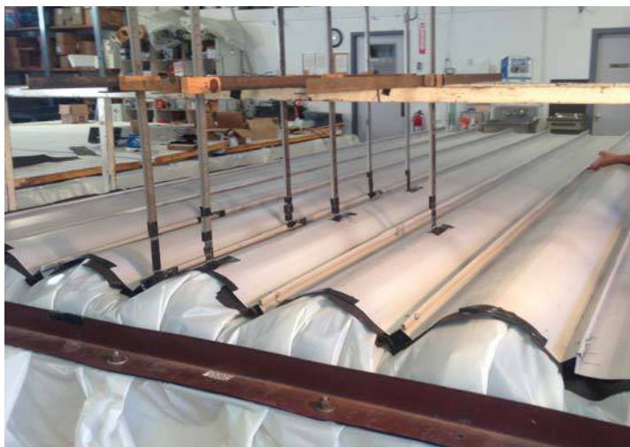
ASTM E 1592 test with pressure being applied.
