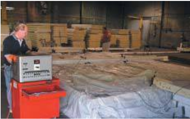
Dan Farabaugh calibrating the sensors before beginning the tests.
