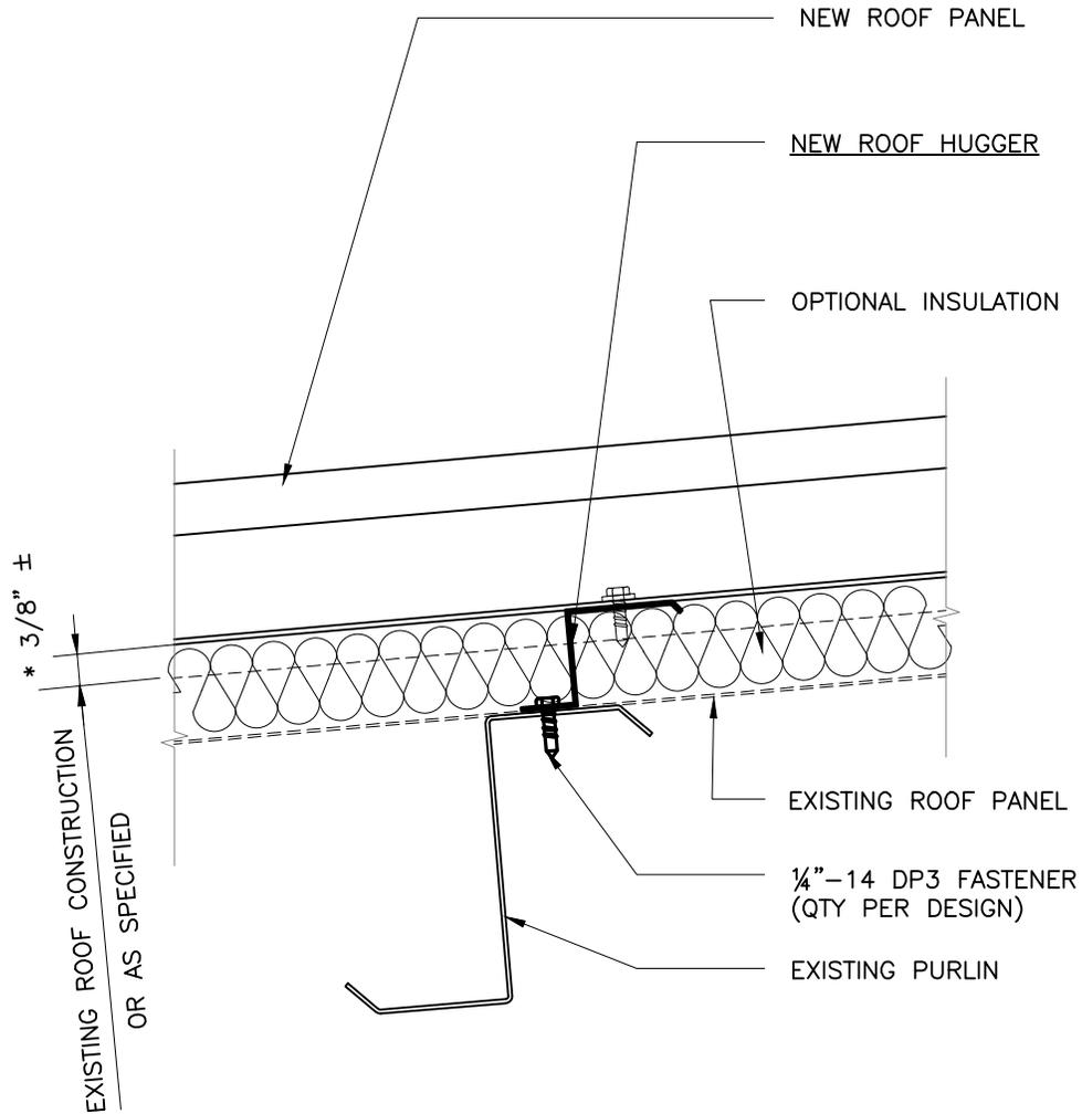
\* ROOF HUGGERS ARE MANUFACTURED TO ALLOW 3/8"-1/2" MIN. ABOVE EXISTING PANEL RIB/SEAM. THIS DIMENSION MAY VARY TO ACCOMMODATE MATERIAL UTILIZATION AND SCRAP REDUCTION ON CUSTOM ROOF HUGGERS
