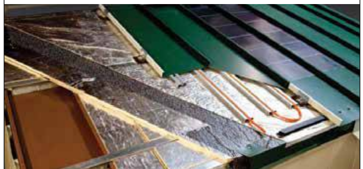
This illustration represents a re-roofing assembly that employs both new insulation, radiant barrier and ASV dynamic ventilation for High-R systems with thermal resistance as much as R-50.
