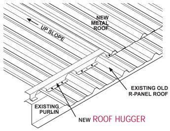
• Installing on Existing Corrugated Panels: ROOF HUGGERS Corru-Fit product for existing 2.50", 2.67" and 2.75" corrugated panels up to 1.25" tall is a 2-part system. A triangular shaped spacer and a 1.5" tall slotted Zee. Spacer/fastener spacing is per engineering design. Call ROOF HUGGER for estimated loads and spacing (subject to review). Lap ends are designed to align and share a common fastener.
